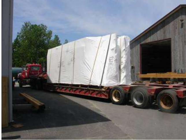
Figure 4: Unity Homes panels sequenced and loaded for shipping
